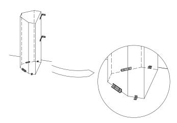
Additionally, the device must be attached to wall in at least two places using dedicated angle bars with one extended arm (the possibility of installing the curtain in the distance from the barrier required by the user).
